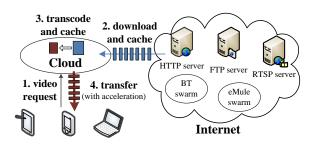
Figure 1: Working principle of Cloud Transcoder.
